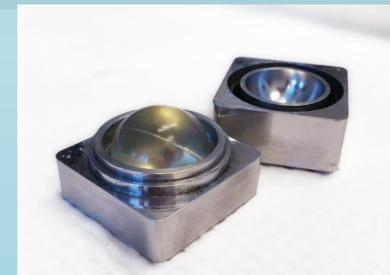
Figure 1. Aluminium mold with one of the  $^{18}\text{F}$ -doped gelatin spheres.
