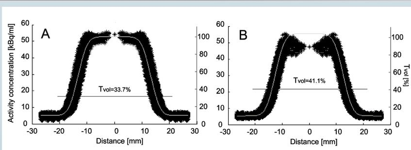
Figure 5. Measured radial activity concentration profile of the large plastic sphere (left) and the large gelatin sphere (right). An isotropic Gaussian PSF was fitted to the experimental data. The grey dotted line represents the background-corrected relative threshold,  $T_{vol}$  [%], which can be used to delineate the true sphere volume.
