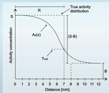
Figure 3. Illustration of the radial activity distribution in a sphere with a radius of 7 mm and a wall thickness of 1 mm.  $S$  is the signal intensity,  $B$  is the background intensity,  $A_z(z)$  is the radial activity concentration profile of a sphere with signal  $S$  surrounded by a background  $B$ , and  $T_{vol}$  is the background-corrected relative threshold (in percent of  $(S-B)$ ).
