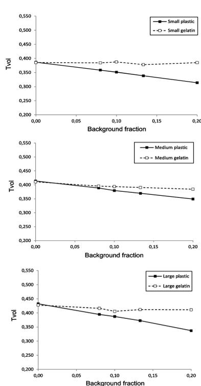
Figure 4.  $T_{vol}$  [%] calculated in spheres of three sizes ( $\phi$ : 27.9 mm, 22.5 mm, and 15.6 mm) as a function of background fraction (BF) with and without non-active walls.
