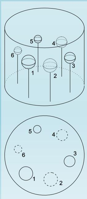
Figure 2. Illustration of the phantom including the placement of the hollow plastic sphere inserts and the gelatin spheres. 1: Large plastic, 2: Large gelatin ( $\phi$ : 27.9 mm), 3: Medium plastic, 4: Medium gelatin ( $\phi$ : 22.5 mm), 5: Small plastic, 6: Small gelatin ( $\phi$ : 15.6 mm).
